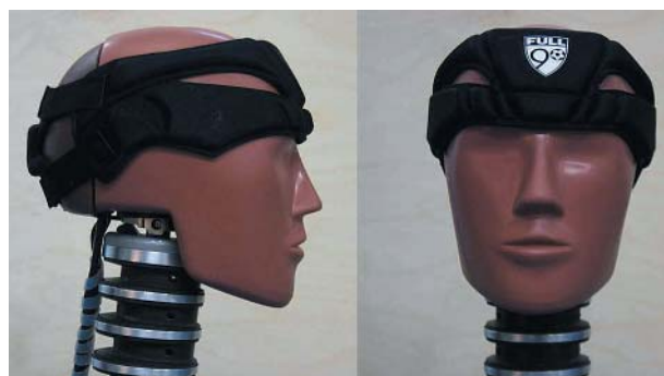
Figure 3 Full90 headgear on Hybrid III.
