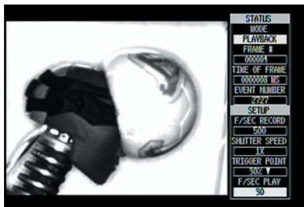
Figure 11 Snapshot from high speed video of 30 m/s ball impact (Full90 headgear).
