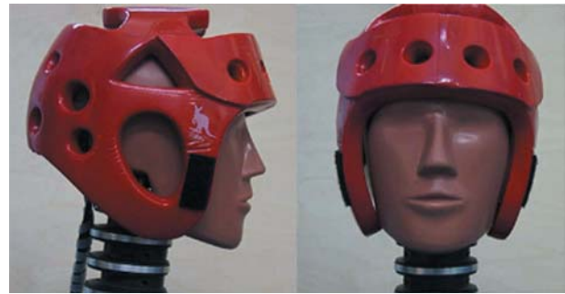
Figure 5 Kangaroo Soccer Headgear on Hybrid III.
